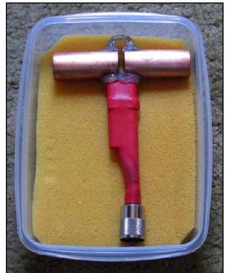
One of the home-made "copper-tube" dipoles, used during "Avon Express". (Photo: GW7BSC)
