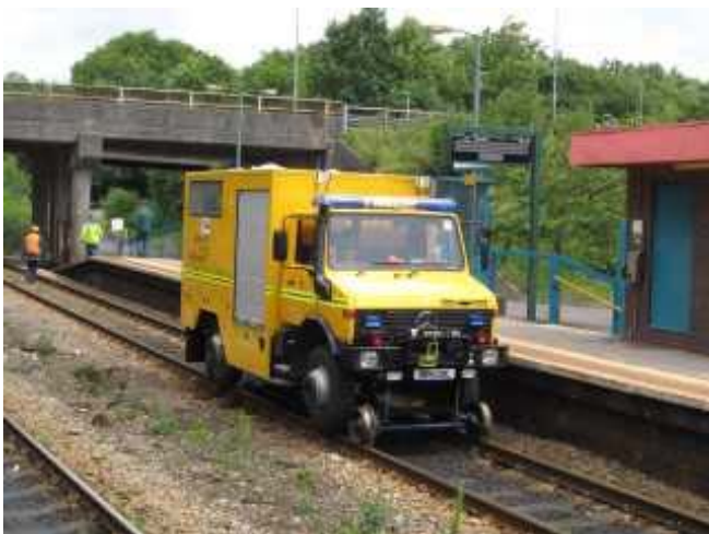
SWFRS “Unimog” Road/Rail vehicle at Lisvane Station, used to transport “casualties” from the train which was in Caerphilly Tunnel. [Photo © GW7BSC]
