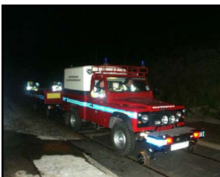
Avon Fire & Rescue Service "Road/Rail" LandRover railed and ready-to-go at the Severn Railway Tunnel Rendezvous Point, Pilning as part of Exercise "Avon Express" which took place on 17/18 September 2005.
